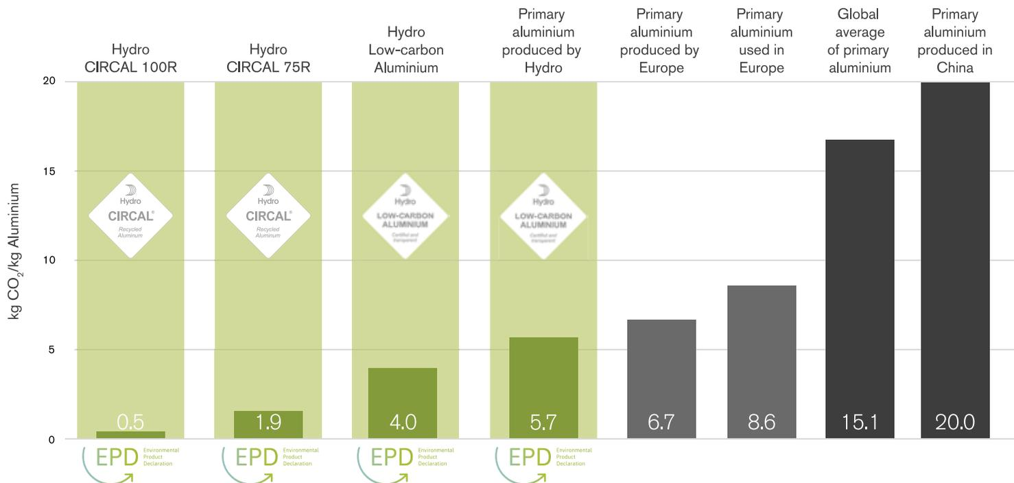
\*75% EoL scrap + 8% process scrap + 11% primary aluminium = 1.9 CO<sub>2</sub>/kg per kg of aluminium
